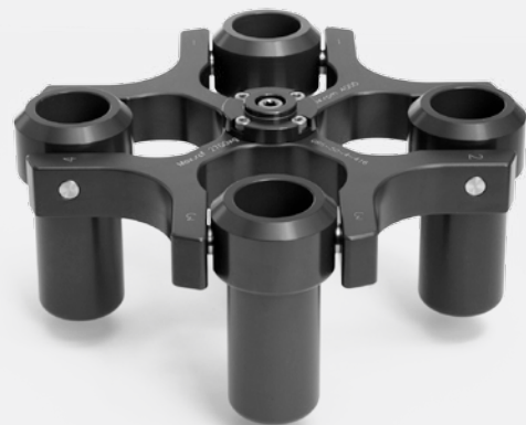
SWING OUT with buckets, with or without adaptors, accepts 15mL to 50mL tubes
